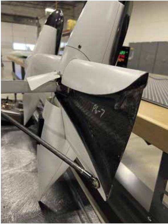
Each pushrod connects to the inner-rear section of its closest wing to achieve the transverse folding and unfolding movements
